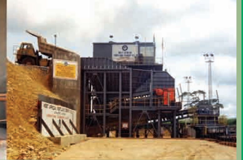
Limestone | Nigeria | In: 1,000mm | Out: -200mm | Capacity: 400TPH
