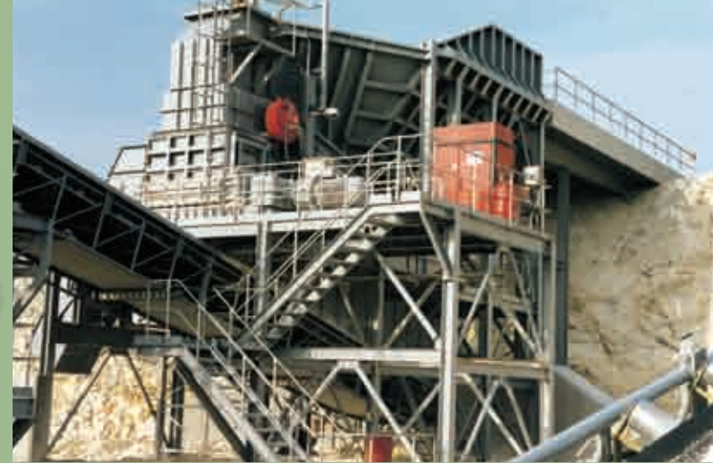
Limestone | Denmark | In: 800mm | Out: -150mm | Capacity: 450TPH
