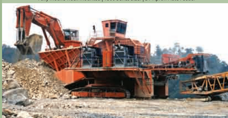
Fully Mobile Track-Mounted | 1300 Series Sizer | D7 Apron Plate Feeder
