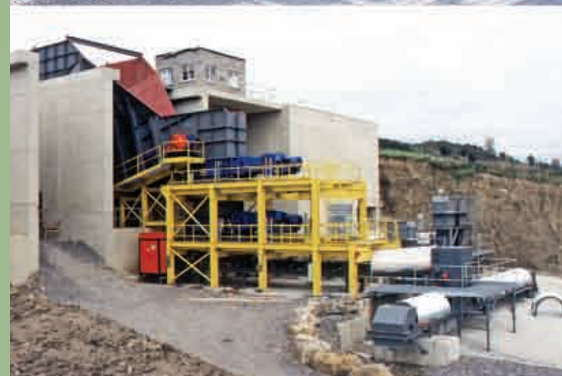
Shale/Limestone/Clay | Ireland | In: 1,000mm | Out: -100mm | Capacity: 500TPH
