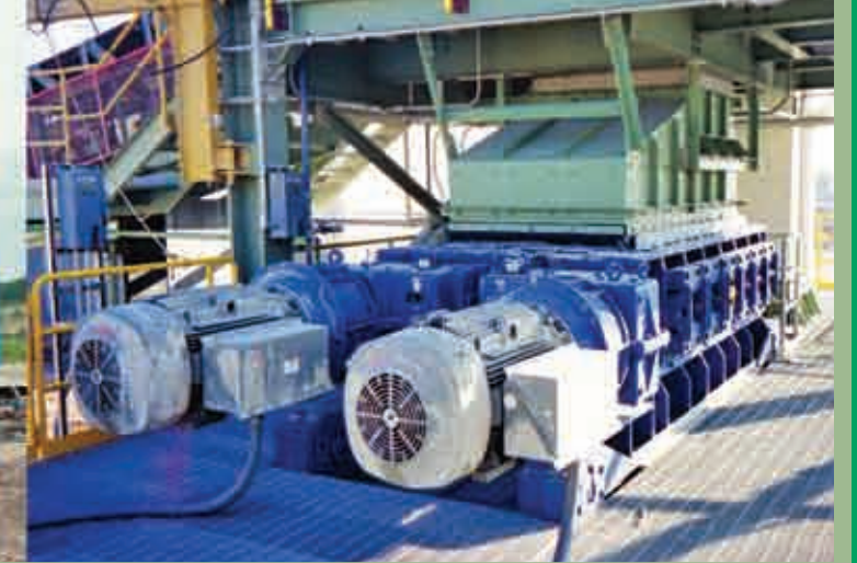
Borax | USA | In: 250mm | Out: -75mm | Capacity: 1,600TPH
