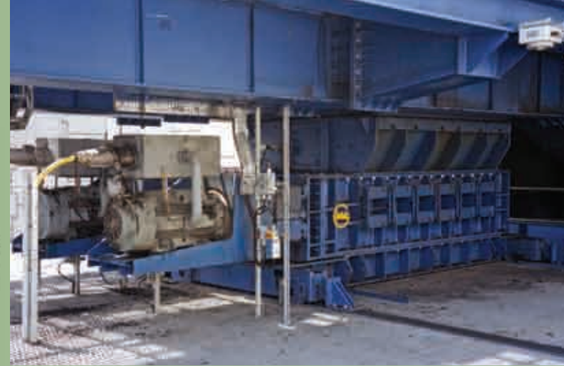
Coal | Colombia | In: 300mm | Out: -50mm | Capacity: 1,600TPH
