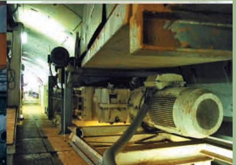
Tunnel Clay/Limestone | Greece | In: 350mm | Out: -200mm | Capacity: 650TPH
