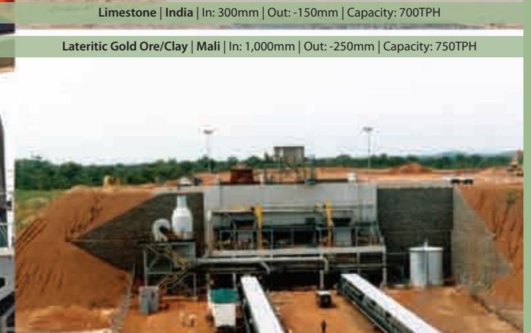
Limestone | India | In: 300mm | Out: -150mm | Capacity: 700TPH
