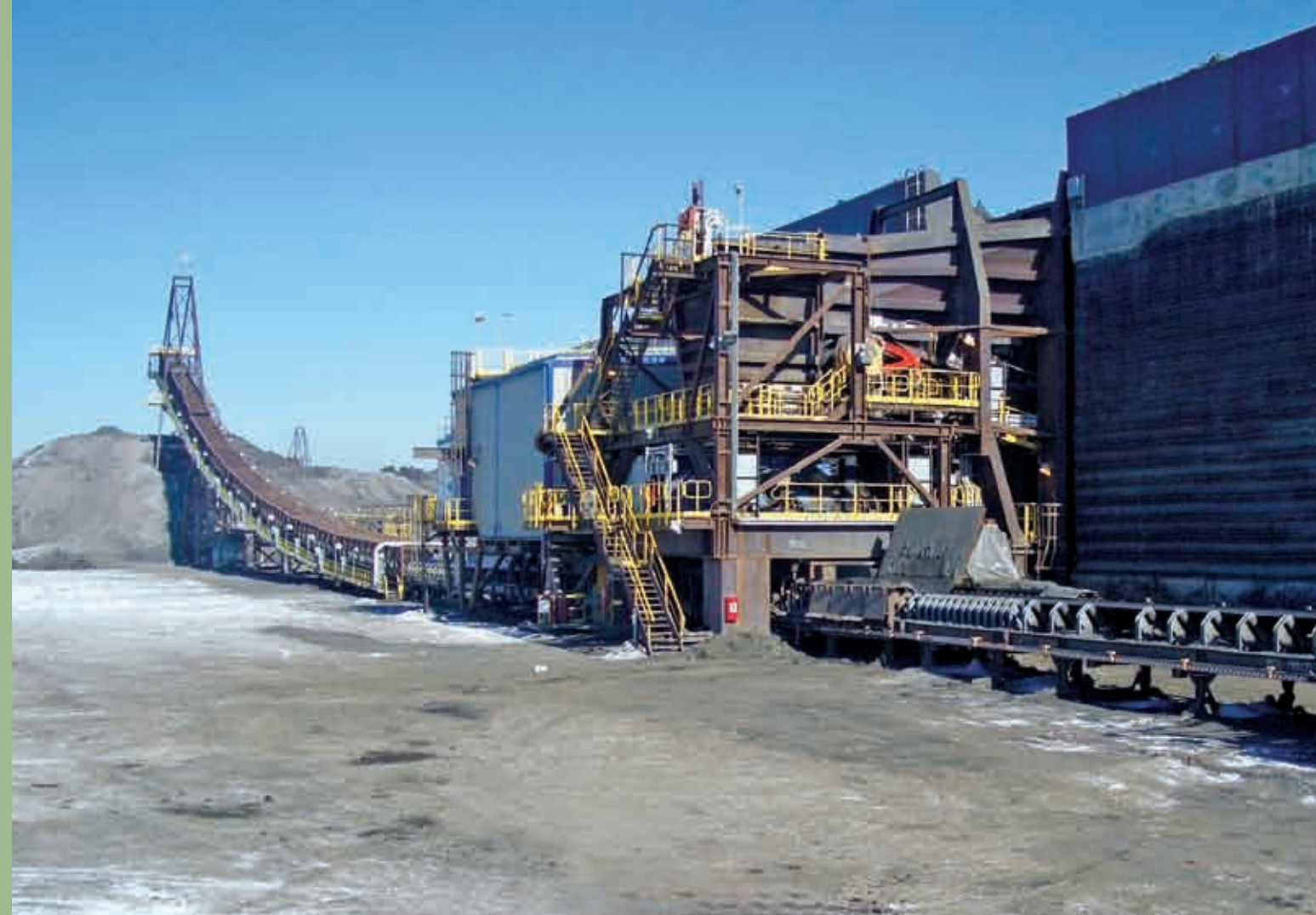
Oil Sands | Canada | In: 3,000mm | Out: -400mm | Capacity: 10,000TPH
