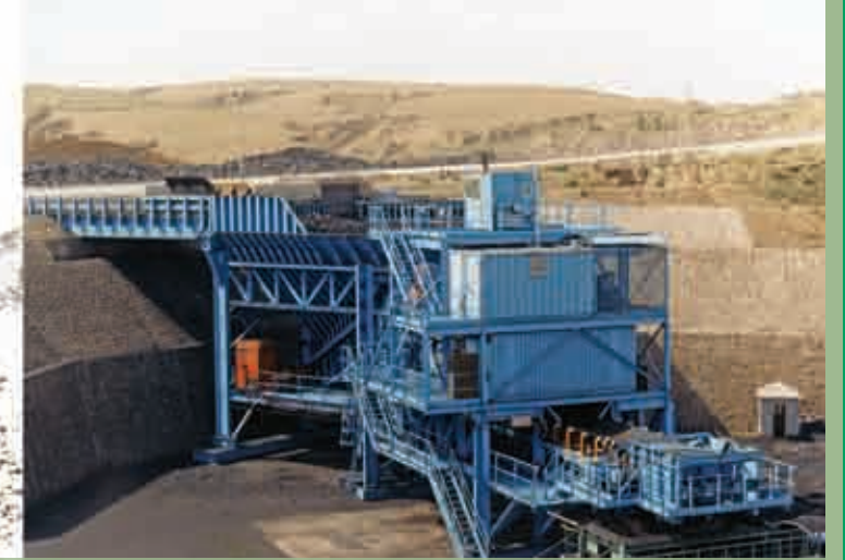
Lignite | China | In: 1,800mm | Out: -300mm | Capacity: 2,500TPH
