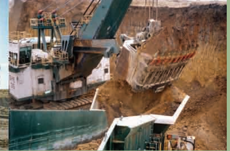
P&H Shovel loading the D9 Plate Feeder, via the 350 Tonne capacity Hopper
