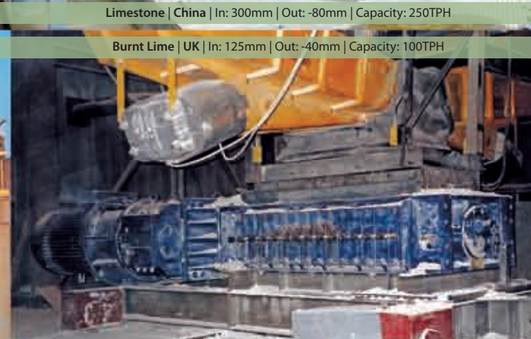
Limestone | China | In: 300mm | Out: -80mm | Capacity: 250TPH
