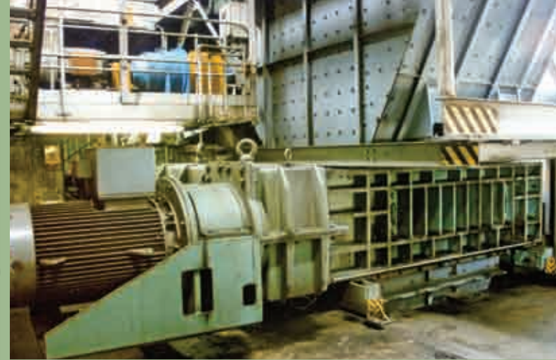
Coal | South Africa | In: 1,000mm | Out: -180mm | Capacity: 900TPH
