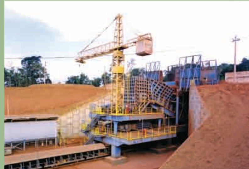
Bauxite | Brazil | In: 1,200mm | Out: -300mm | Capacity: 3,000TPH
