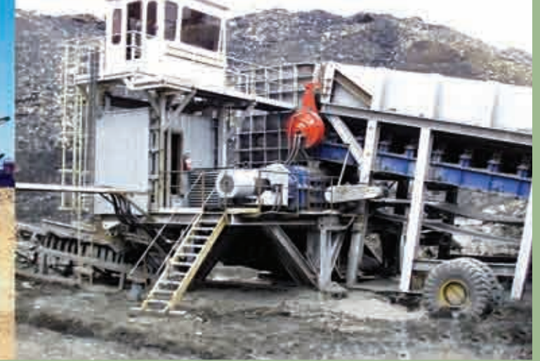
Overburden | Canada | In: 1,500mm | Out: -250mm | Capacity: 2,000TPH
