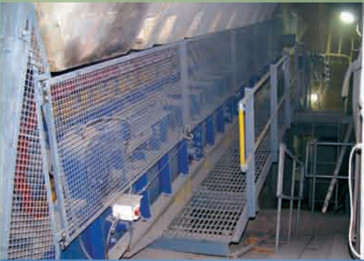
D9 Apron Plate Feeder forming part of the Fully Mobile Slewing Sizer Station
