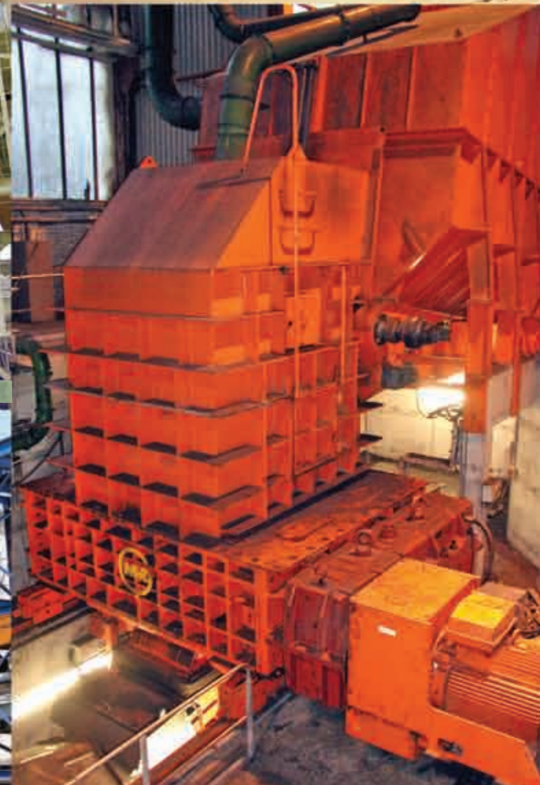
Carbon Anodes | Norway | In: 1,600mm | Out: -350mm | Capacity: 70TPH
