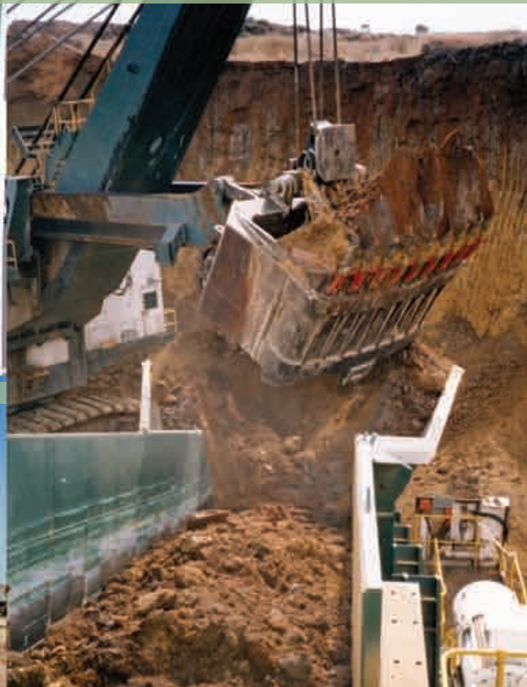
D9 Apron Plate Feeder with electro-mechanical drive
