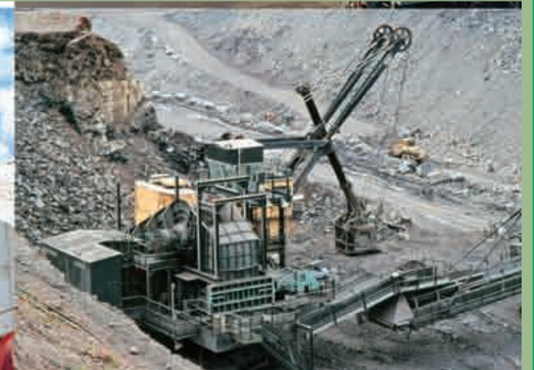
Overburden | UK | In: 1,500mm | Out: -350mm | Capacity: 1,000TPH
