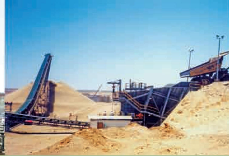
Mineral Sands | South Africa | In: 1,500mm | Out: -300mm | Capacity: 1,500TPH
