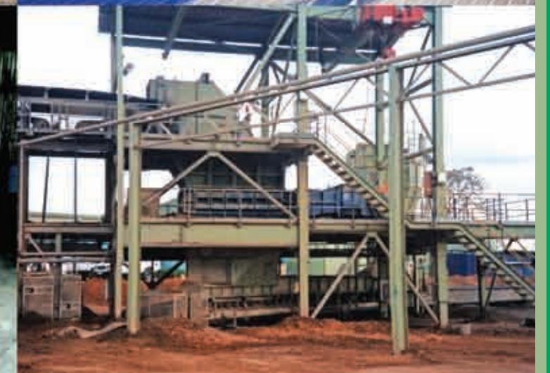
Gold Ore | Guinea | In: 350mm | Out: -80mm | Capacity: 1,500TPH
