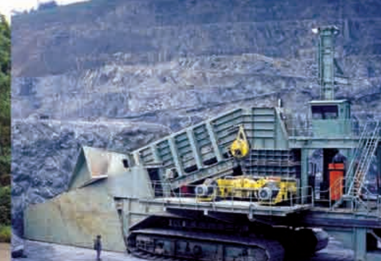
Semi-Mobile | 1250 Series Sizer | D7 Apron Plate Feeder
