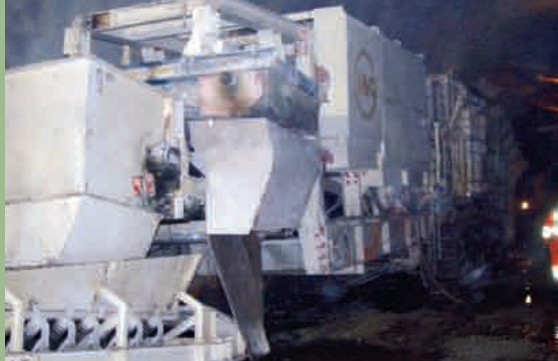
Fully Mobile Track-Mounted | 850 Series Sizer | D7 Apron Plate Feeder
