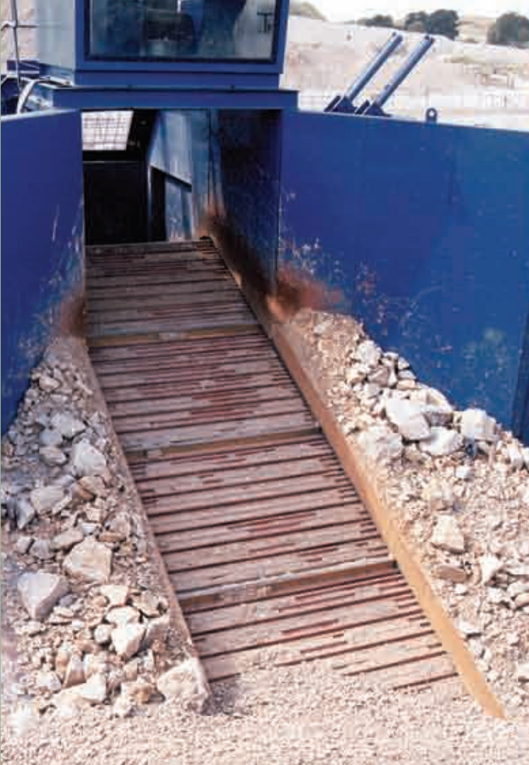
D7 Apron Plate Feeder with Fines Retrieval System
