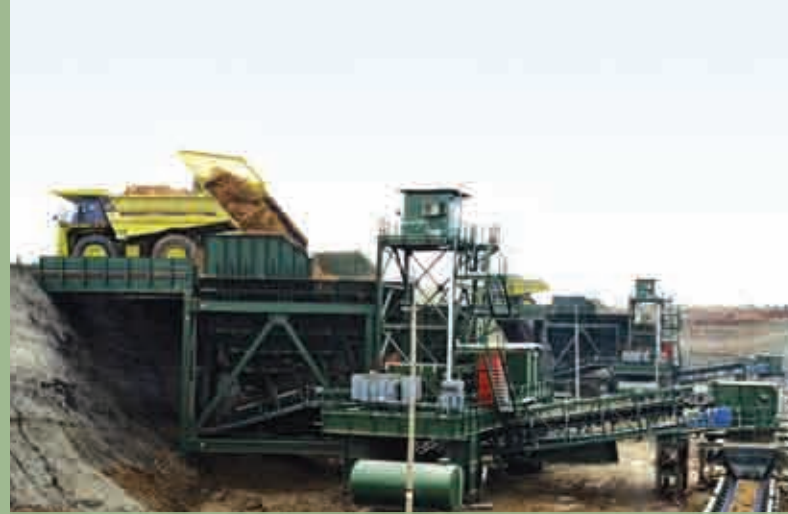
Overburden | Thailand | In: 1,200mm | Out: -400mm | Capacity: 6,500TPH
