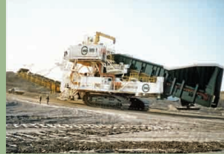
Sizer Station negotiating a +10% gradient
