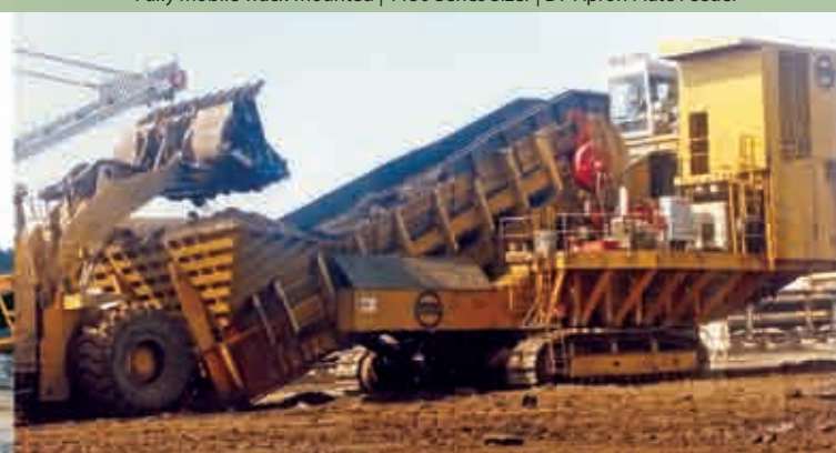
Fully Mobile Track-Mounted | 1150 Series Sizer | D7 Apron Plate Feeder
