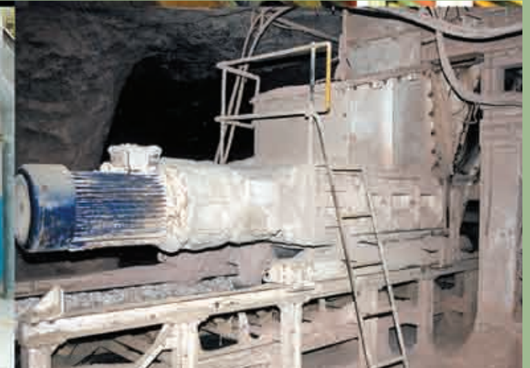
Gypsum | UK | In: 150mm | Out: -40mm | Capacity: 300TPH
