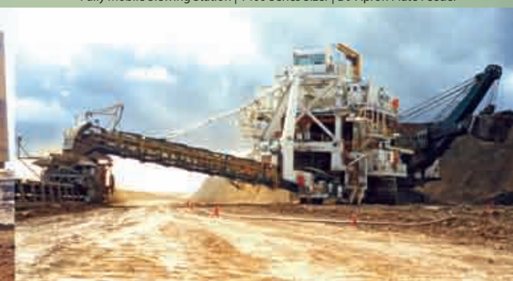
Fully Mobile Slewing Station | 1400 Series Sizer | D9 Apron Plate Feeder
