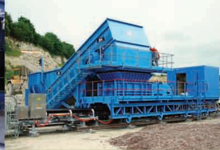
Chalk | Belgium | In: 800mm | Out: -250mm | Capacity: 500TPH
