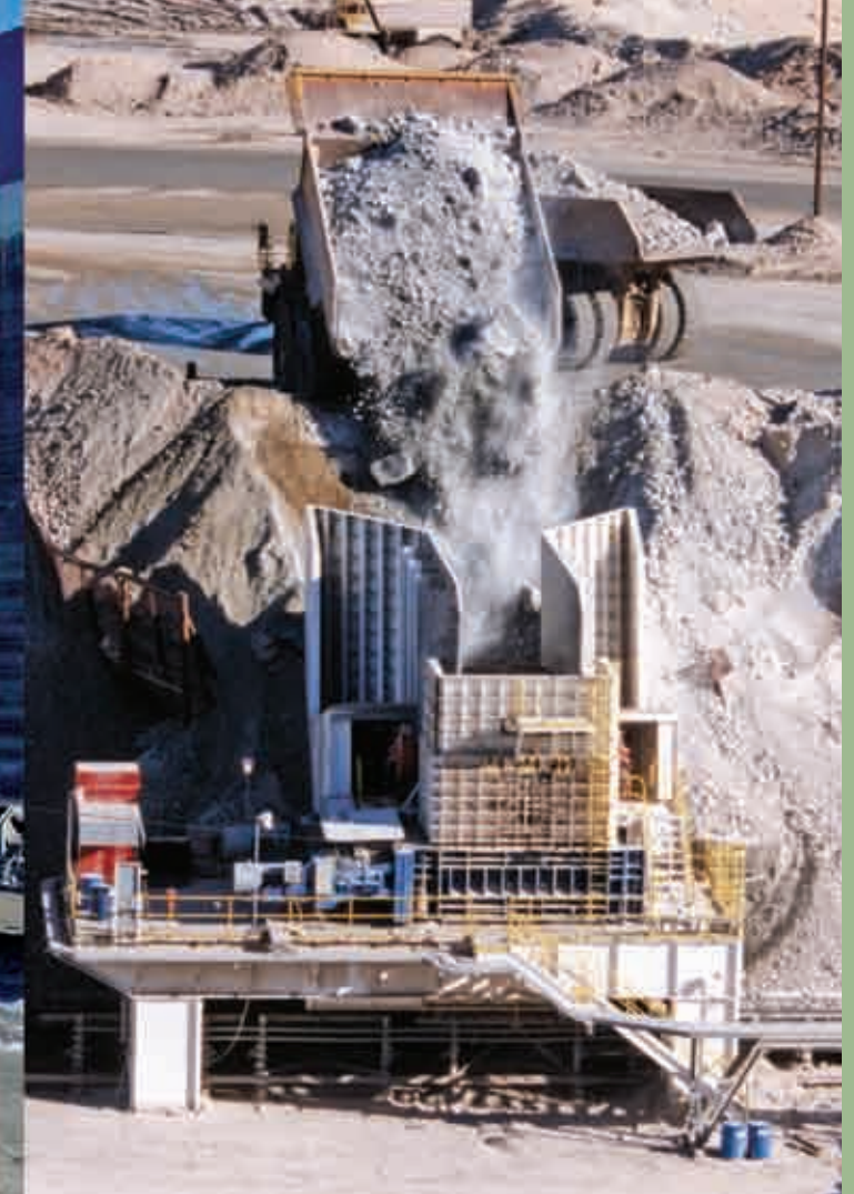
Overburden | Colombia | In: ROM | Out: -450mm | Capacity: 10,000TPH
