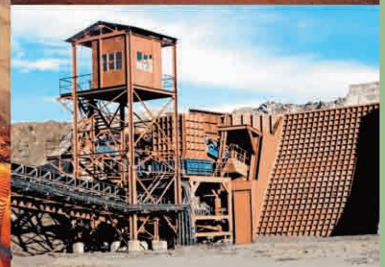
Limestone | India | In: 300mm | Out: -150mm | Capacity: 700TPH
