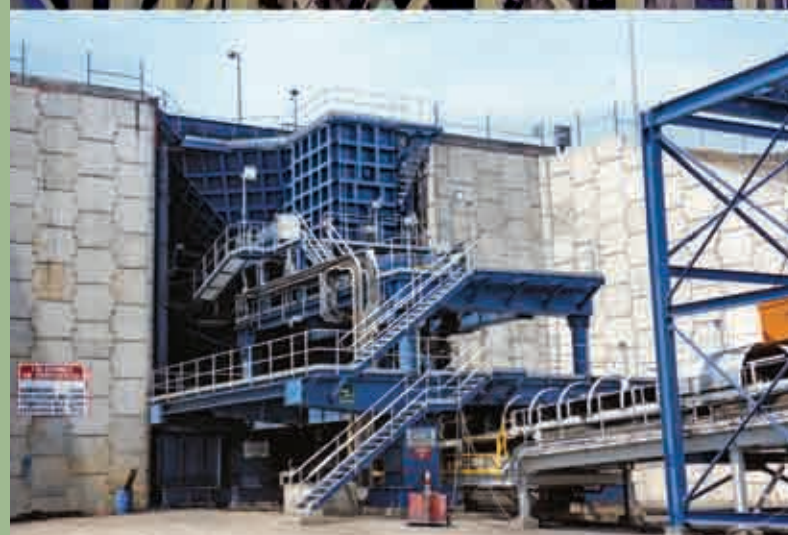
Coal | Colombia | In: 300mm | Out: -50mm | Capacity: 1,600TPH
