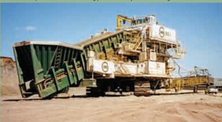
D9 Apron Plate Feeder forming part of the Fully Mobile Slewing Sizer Station
