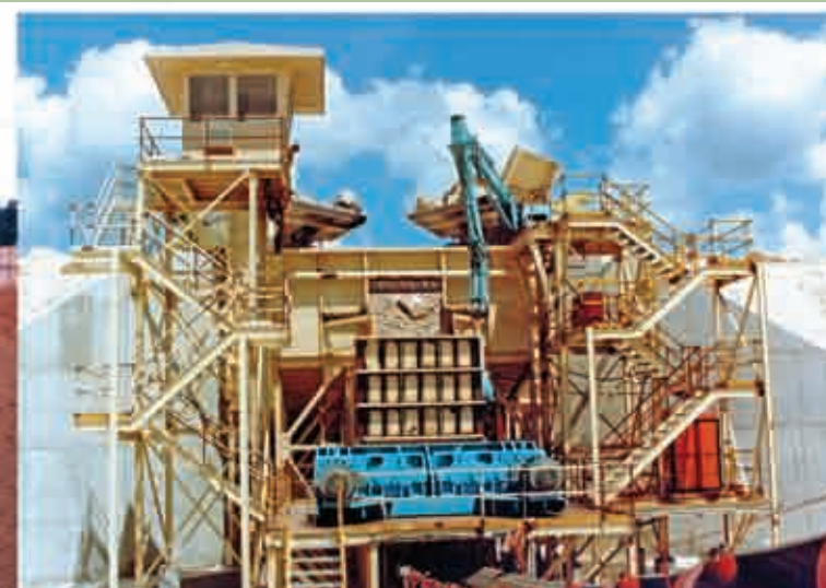
Limestone | Mexico | In: 1,250mm | Out: -300mm | Capacity: 2,000TPH
