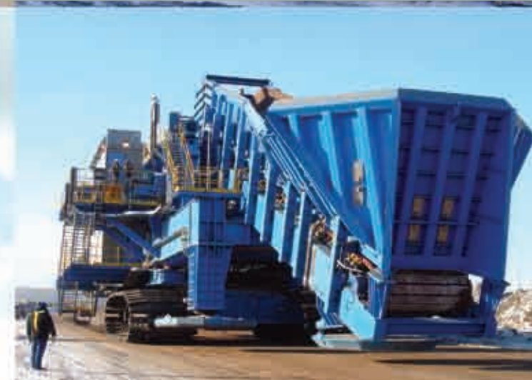
Fully Mobile Slewing Station | 1500 Series Sizer | D9 Apron Plate Feeder
