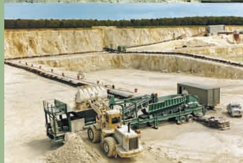
Chalk | UK | In: ,500mm | Out: -300mm | Capacity: 600TPH
