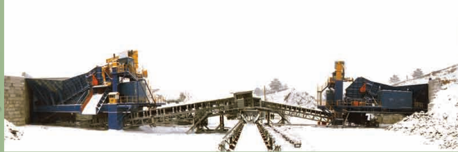
Overburden | Russia | In: 1,200mm | Out: -350mm | Capacity: 3,500TPH
