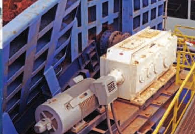
D7 Apron Plate Feeder with electro-mechanical drive
