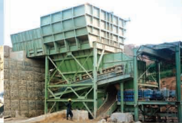
Quartzite | Ghana | In: 500mm | Out: -100mm | Capacity: 300TPH
