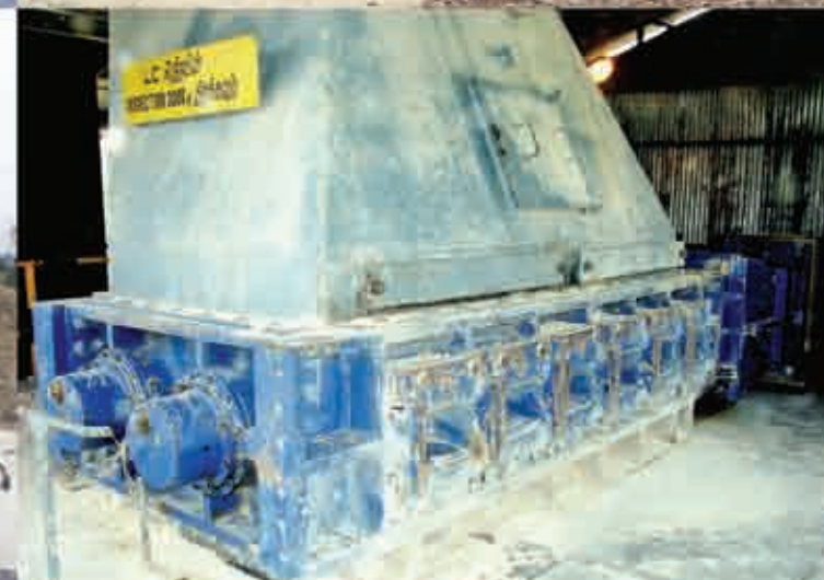
Clay/Limestone | India | In: 350mm | Out: -90mm | Capacity: 750TPH
